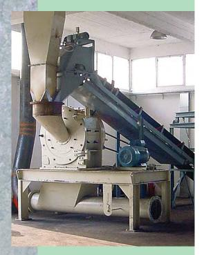
Impact Mill with hot gas system for drying and pneumatic transport of ground product
