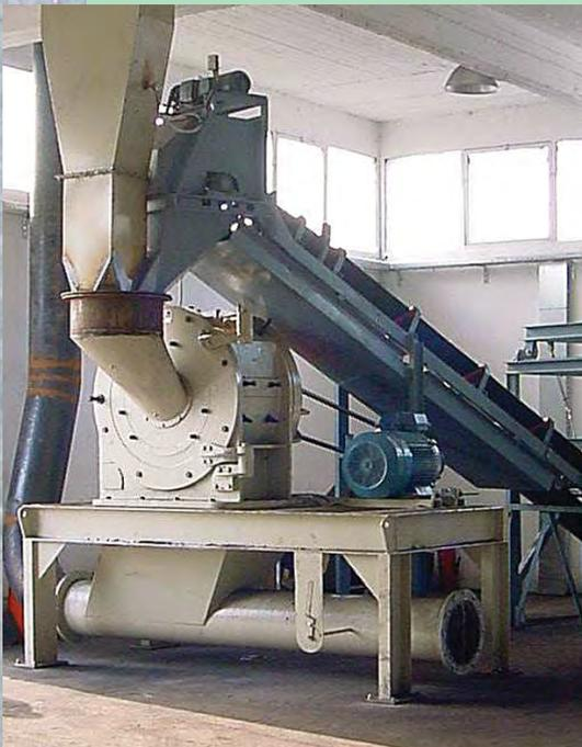
*Impact Mill with hot gas system for drying and pneumatic transport of ground product*
