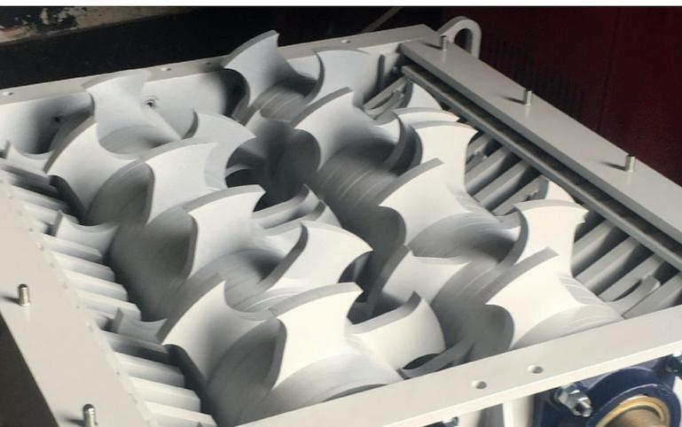
The **LUMP BREAKER model RIP** is designed to be used as primary crusher for materials agglomerated in lumps or sods, such as clays, bentonite, chemical products, fertilizers, casting earth.
