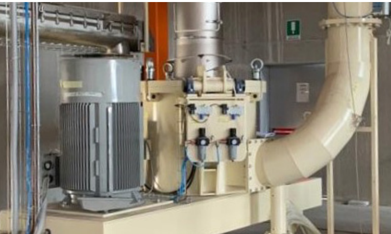
Grinding plant of chemicals with PPS-1000 TX
